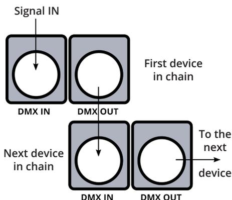
**Step 1:** Connect the male connector of the DMX cable to the female connector (output) on the controller.
