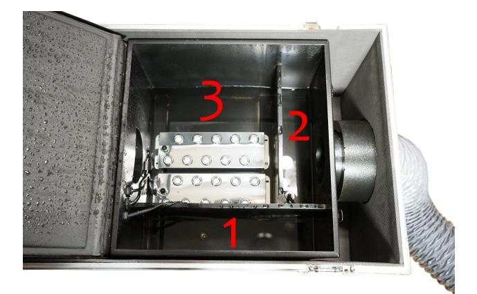
The S-LOW FOG contains 3 different tanks. You can fill with water all of them, as they are connected. As the fog machine operates, the water level in tank 3 reduces. An electric pump then will
